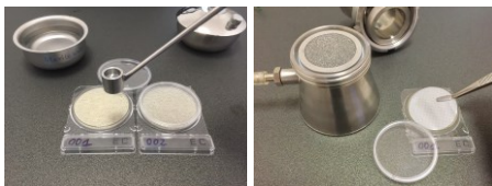
Activation and placing Membrane Filter after sample filtration with the portable LetzTEST Membrane Filtration Kit
